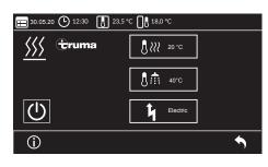
To activate / deactivate the heating system, press lightly on the "On/Off" icon .
