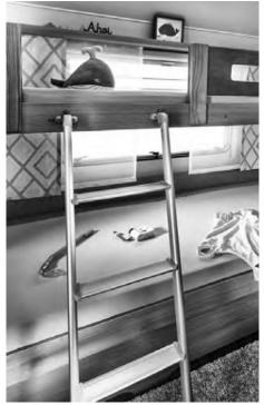
The maximum load for the upper bunk bed is 75 kg.
