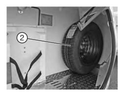
• The spare tyre with mount (model/series-specific, optional extra) ② can be stored at the front of the caravan by the gas bottle container. (The mount will only be included in the scope of delivery if the spare tyre is fitted at the factory.)
