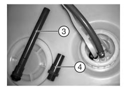
The water can be emptied from the tank by unscrewing the overflow pipe 3.
